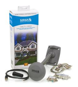
The SIRIUS CATV Home Distribution Kit (p/n 14250) lets you send a SIRIUS satellite radio signal to any room in your home with a cable TV outlet. The kit includes an all-weather outdoor antenna, 2 diplexer signal splitters, and the necessary adapter to supply signal to a SIRIUS satellite radio. As with the Satellite TV Distribution System above, RG6/F cabling must be added to complete the antenna/combiner installation.
